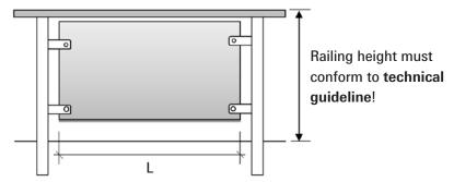
**Hinweis:** If the types of glass and the dimensions listed in Table B are used, only static structural proof calculations are required.
