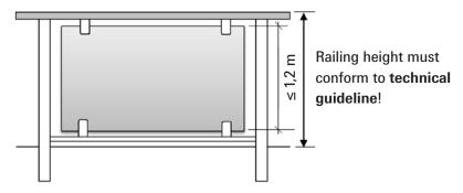
6.3 Balustrade with horizontal bars (protection against falling is provided solely by sufficiently strong handrails and knee-height bars)
