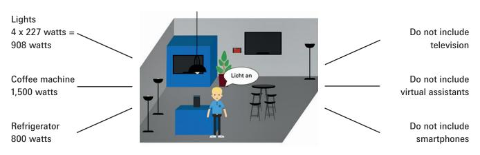
Electrical appliances: 908 watts + 1,500 watts + 800 watts = 3,208 wattsReserve capacity:  $3,208 \text{ watts} \times 10 \% = 321 \text{ watts}$
